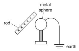
The earth connection is removed and then the rod is removed.
